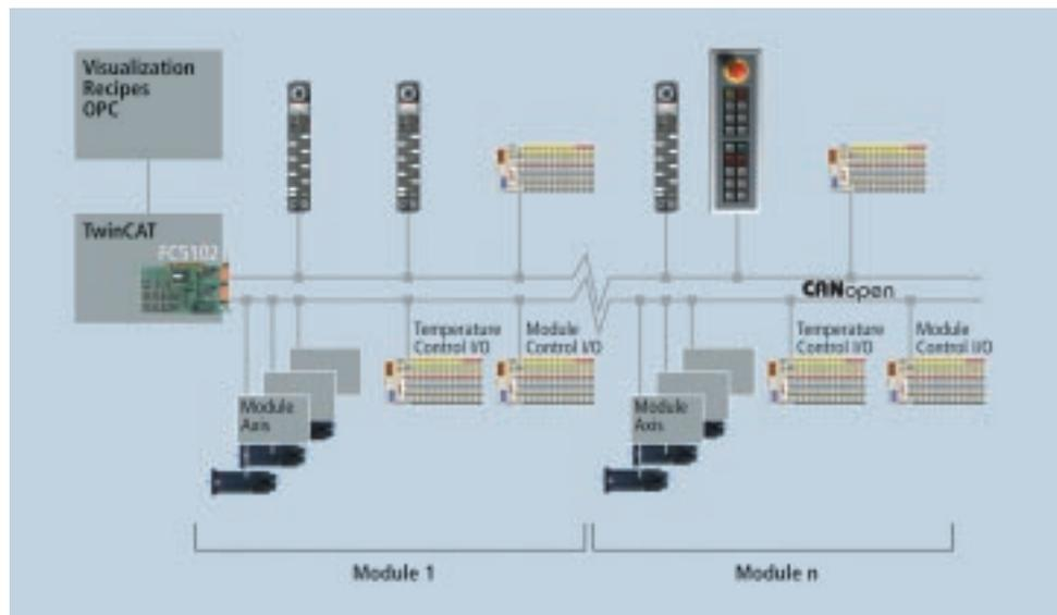
sists of the stand alone Compact Box, the Coupler Box and the Extension Box modules. The modules meet the Protection Class IP 67 and are wired using either premolded cord sets or field-wireable connectors. Together with the IP67 Fieldbus Box Mattson has selected Beckhoff's IP20 Bus Terminal series. The CANopen bus coupler supply up to 64 electronic terminal blocks for any type of signal. Different volt-
