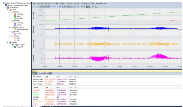
The mover behaves much more poorly than the straight sections. This is to be expected, the physics of motion change when rotating vs travelling in a straight line. The important part is that there are no high frequency oscillations in the curves, if the mover oscillates in the curves, the filters must be re-adjusted so that the mover does not oscillate in the curve.
