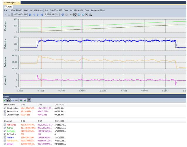
With the velocity loop tuned the Position control loop can now be tuned.
