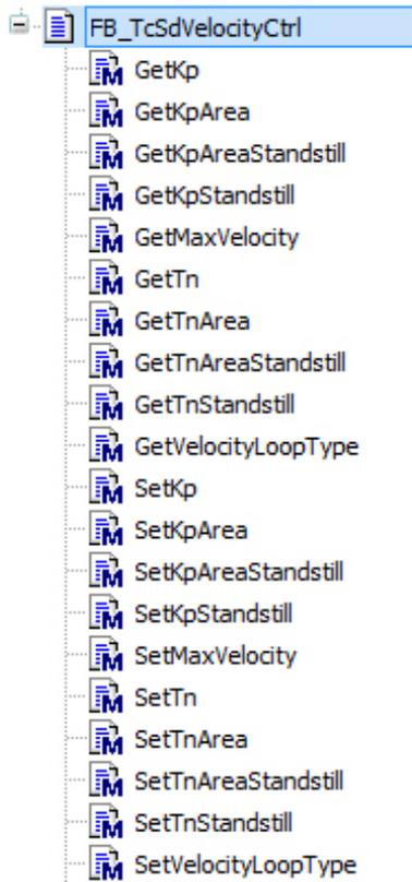
The FB\_TcSoftDrive contains sub blocks, one for each parameter set and these blocks contain methods to read and write individual parameters.
