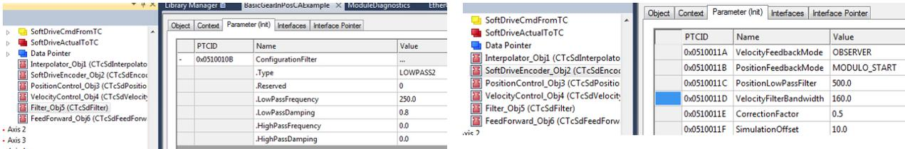
Start the Scope of the Axis, Enable the Axis and monitor the oscillations. **Depending on the load these Oscillations can be extremely loud > 80dB.** Increase/decrease the filters as necessary until the mover settles nicely without significant oscillations.
