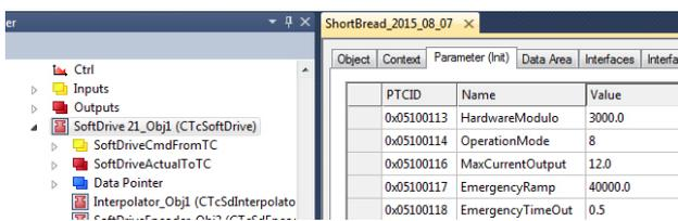
The Operation mode of the axis must be set back to Mode 8 to allow Position Control
