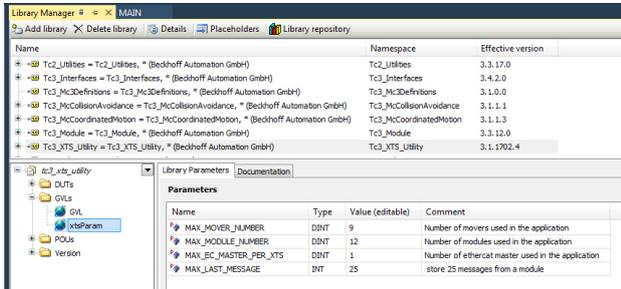
The XTS\_Utilities library contains a block FB\_XTSUnit. This block will obtain ALL XTS module status and diagnostic information as well as all Soft Drive Mover Parameters. It is also possible to write any value to any Soft Drive Parameter of any mover. To use this block simply add the XTS\_Utilities Library, adjust the library's Global Parameters to match the configuration of the XTS.
