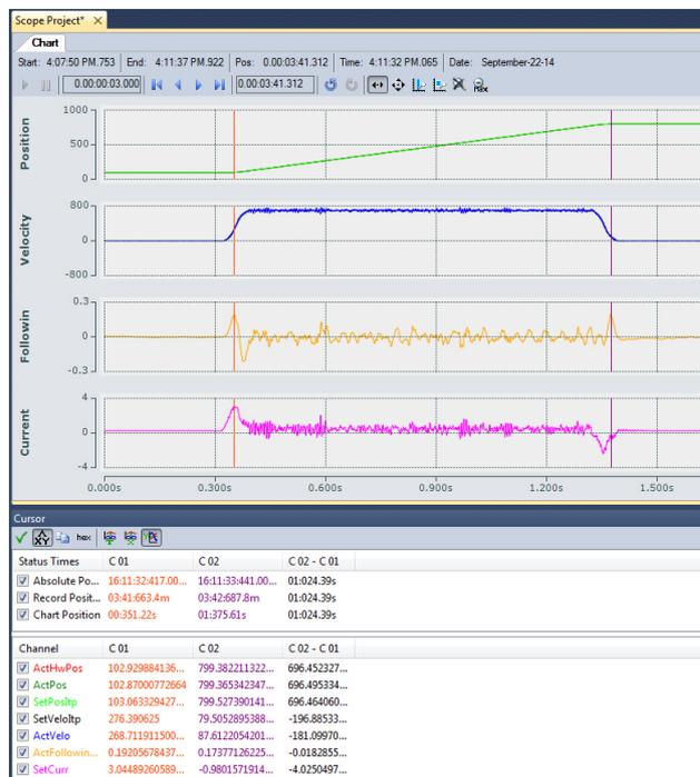
If the mover requires tuning values outside the recommended settings, the mover will not be able to attain and hold position and the mechanical construction of the tooling mounted to the mover should be re-designed. Pay particular attention to Project Planning guide which describes the physics and effects of various loads on the mover.
