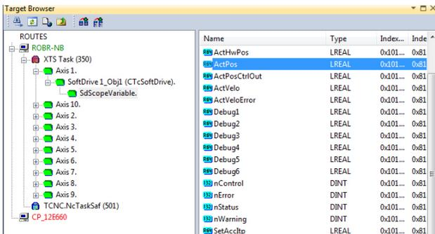
To select the appropriate values use the Target Browser (TwinCAT must be in Run Mode). Soft Drive Variables are found under the Axis SoftDrive\_Obj (CTcSoftDrive). If the sdScopeVariables are NOT present, check that the XTS Task is correctly configured on Port 350 or higher.
