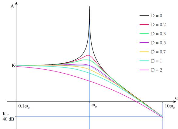
A damping factor of 0.8 provides a reasonable response and is generally sufficient. Damping factors less than 0.5 should not be used.
