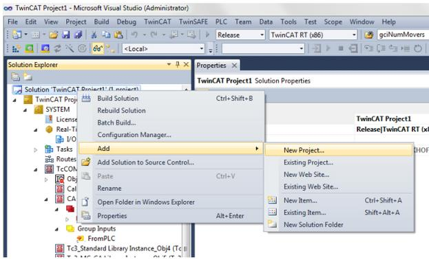
To scope the values add a TwinCAT measurement project to the Solution.
