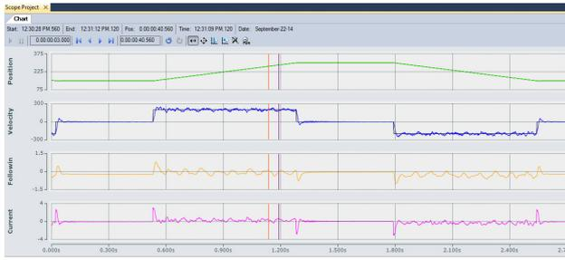
Here the a velo step sequence is implanted with a 0.75 second driving time
