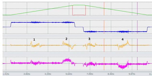
Depending on the location of the center of gravity on the mover and the orientation of the XTS It is much more difficult to tune the system in the curves and it simply will not behave as well as when in the straight sections.
