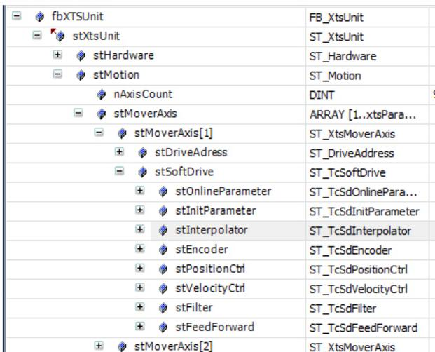
The FB\_XTSUnit block contains the structure stMotion, stMotion contains the number of movers (axis) and an array with all of the movers information. stMoverAxis [1] contains all the information about the first mover axis.
