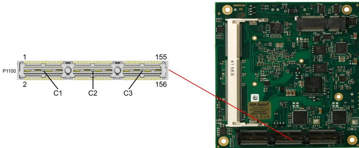
Pinout PCI104-Express connector (type 2):
