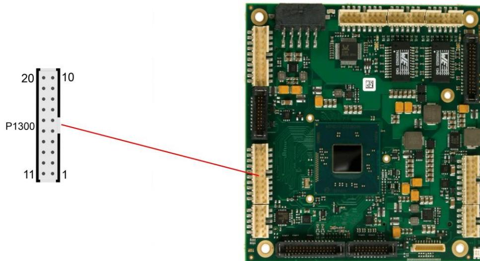
Pinout GPIO connector:
