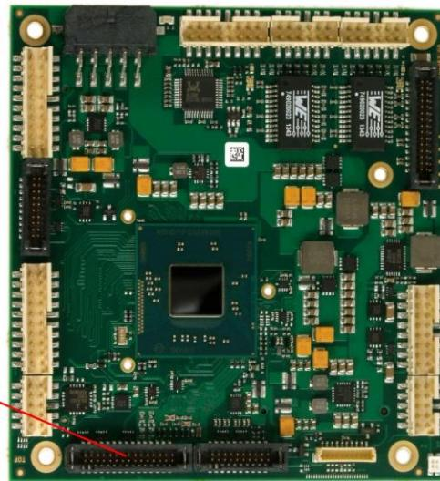
Pinout 2x15 connector DVI/HDMI/VGA:
