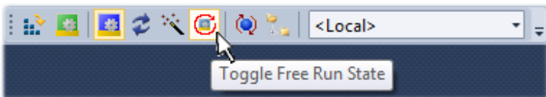
Fig. 92: TwinCAT can also be switched to this state by using a button (TwinCAT 3)
