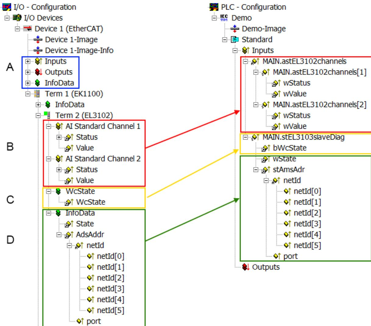
Fig. 133: Basic EtherCAT Slave Diagnosis in the PLC
