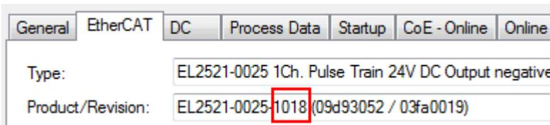
Fig. 106: Installing EthetCAT terminal with revision -1018
