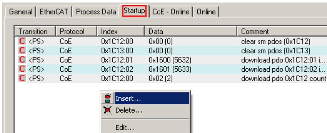
Fig. 16: Startup list in the TwinCAT System Manager
