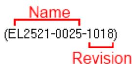
Fig. 83: Identifier structure
