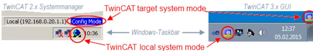
Fig. 101: Differentiation local/target system (left: TwinCAT 2; right: TwinCAT 3)
