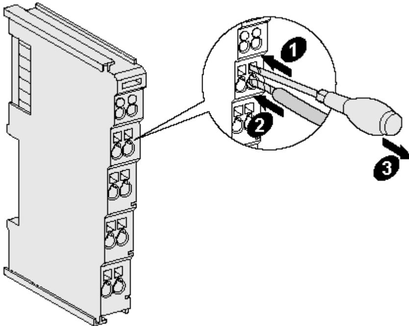
Fig. 26: Mounting a cable on a terminal connection
