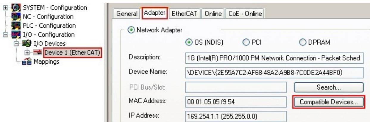
Fig. 78: EtherCAT device properties(TwinCAT 2): click on “Compatible Devices...” of tab “Adapte””
