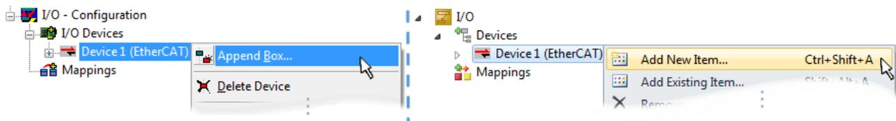
Fig. 95: Appending EtherCAT devices (left: TwinCAT 2; right: TwinCAT 3)
