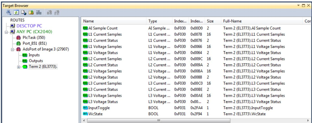
Fig. 153: Direct access to PDOs of the terminal by ScopeView
