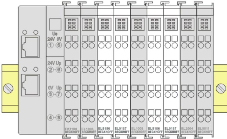
Fig. 29: Correct positioning
