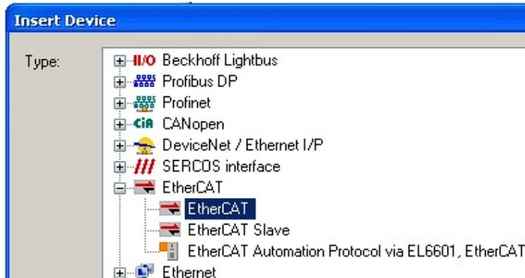
Fig. 92: Selecting the EtherCAT connection (TwinCAT 2.11, TwinCAT 3)
