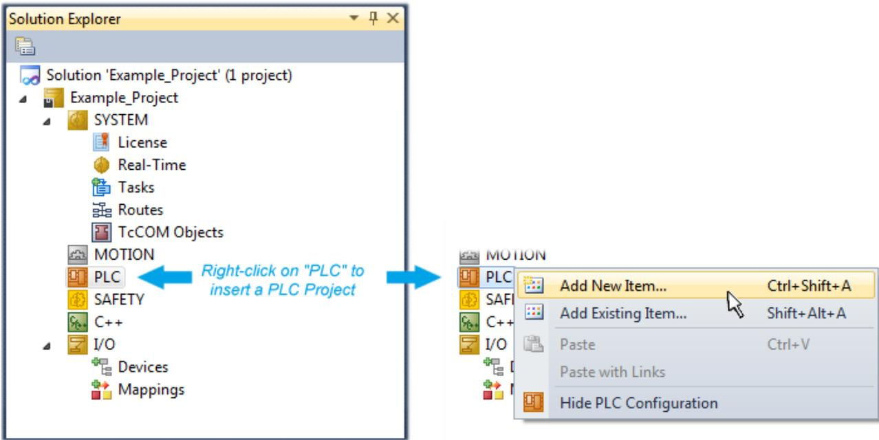
Fig. 61: Adding the programming environment in “PLC”
