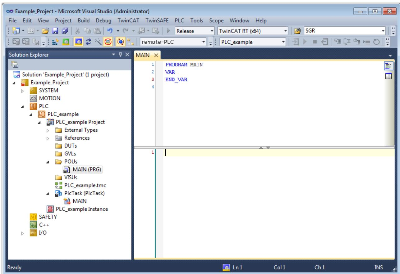
Fig. 63: Initial “Main” program of the standard PLC project
