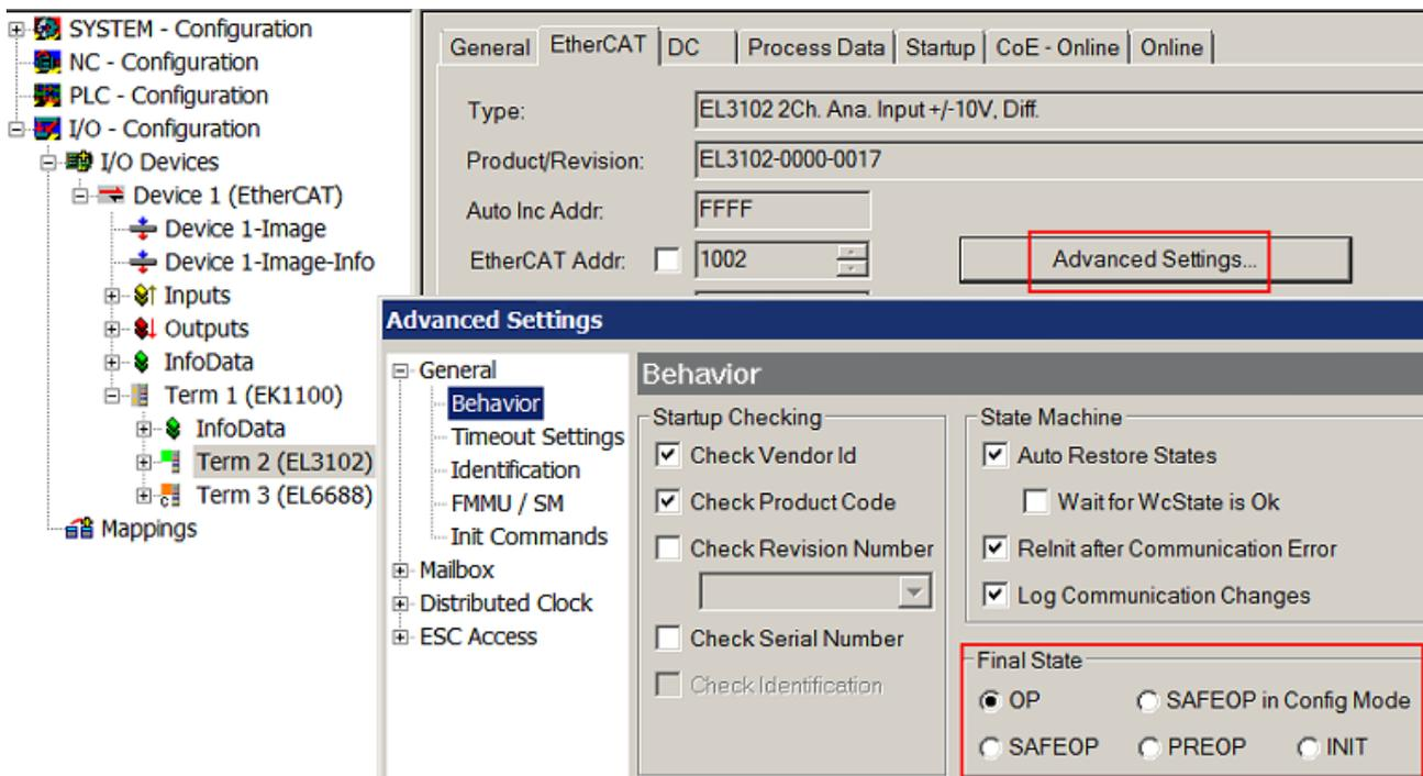
Fig. 137: Default target state in the Slave
