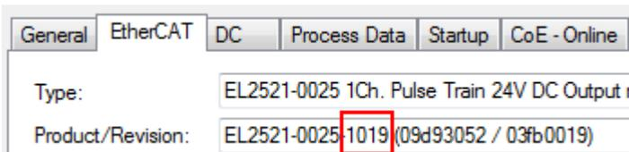
Fig. 107: Detection of EtherCAT terminal with revision -1019
