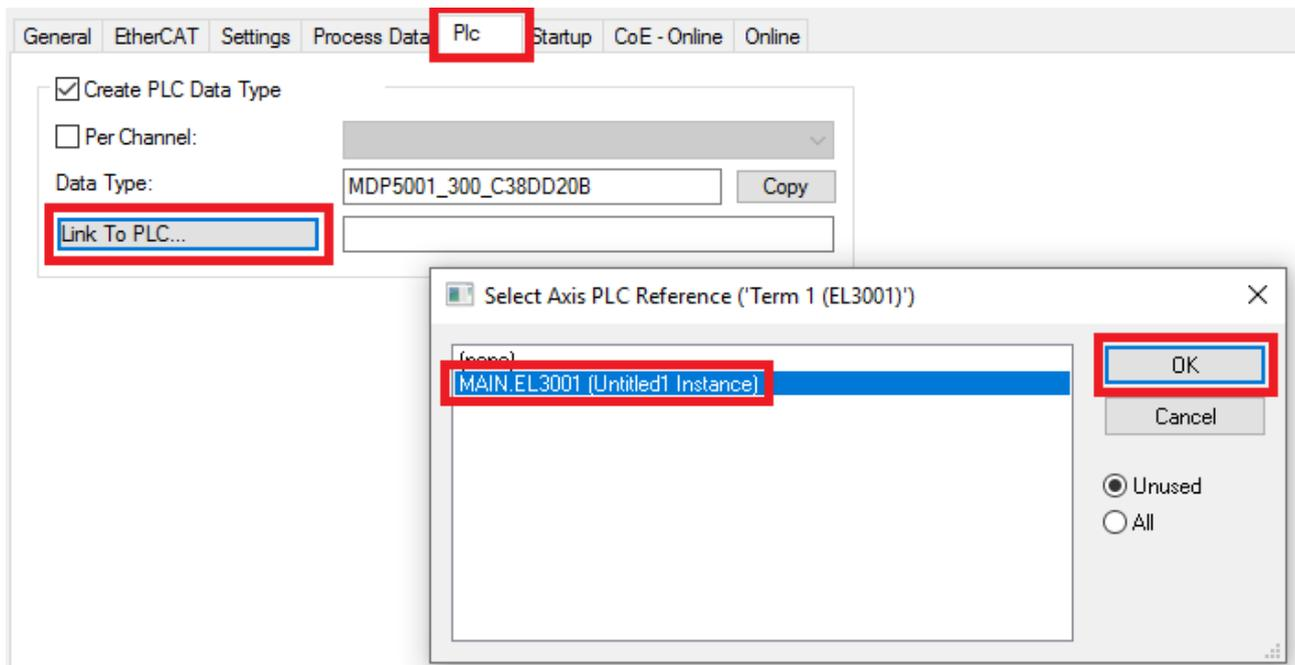
Fig. 72: Linking the structure
