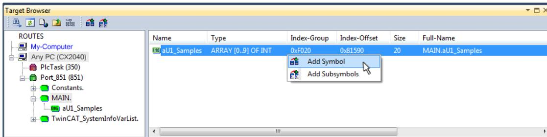
Fig. 150: Appending the variable "aUI\_Samples" below "axis" within the scope project of the solution explorer
