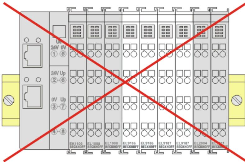
Fig. 30: Incorrect positioning
