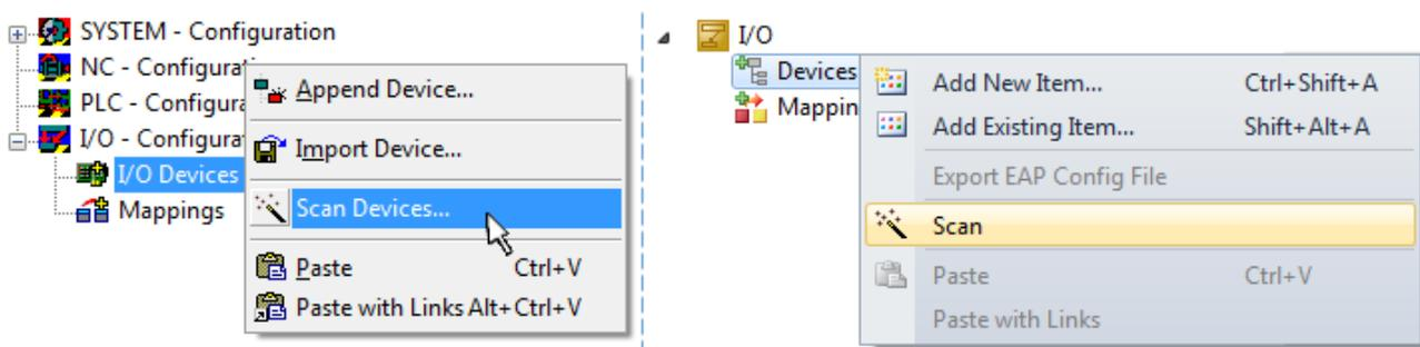
Fig. 102: Scan Devices (left: TwinCAT 2; right: TwinCAT 3)
