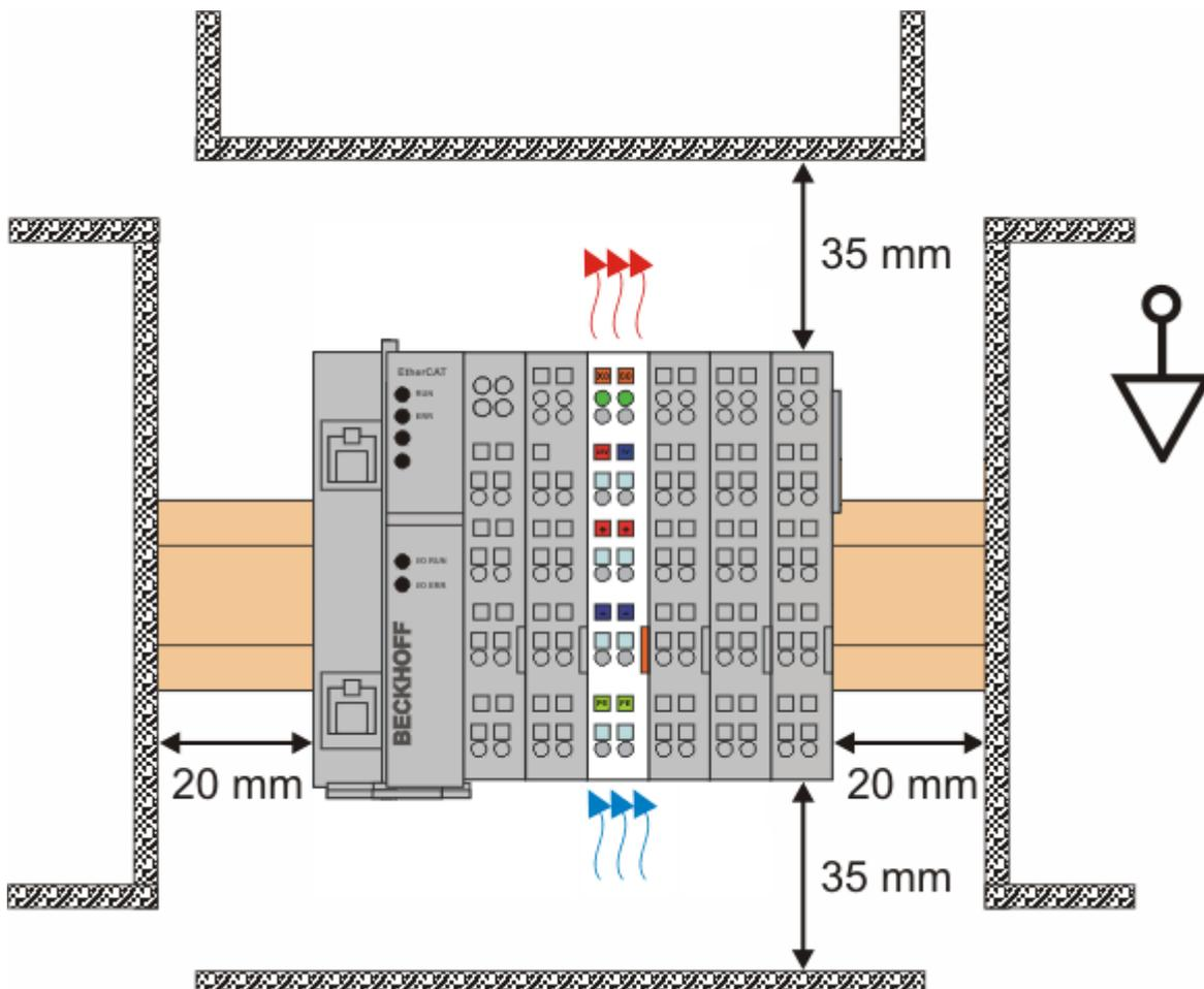
Fig. 27: Recommended distances for standard installation position
