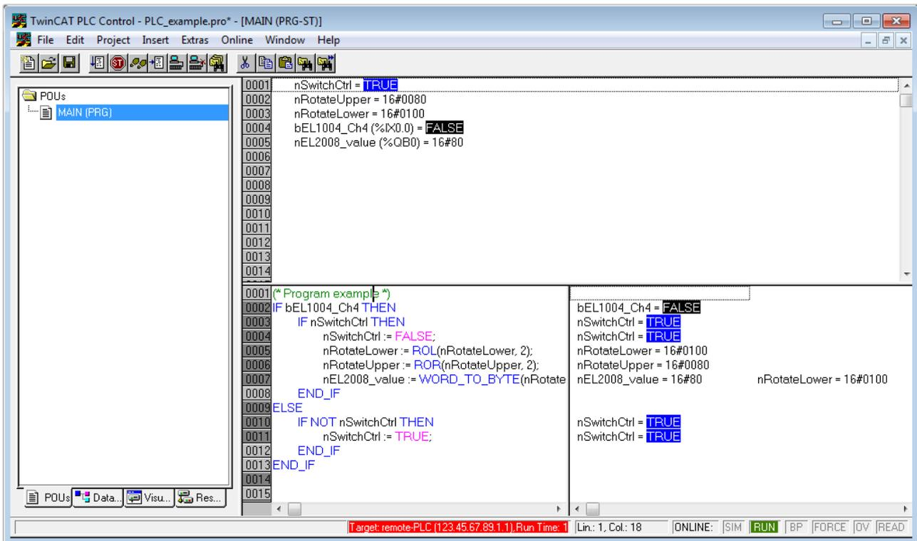
Fig. 51: PLC Control logged in, ready for program startup
