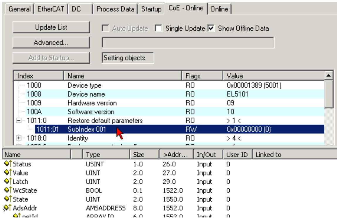
Fig. 205: Selecting the *Restore default parameters* PDO
