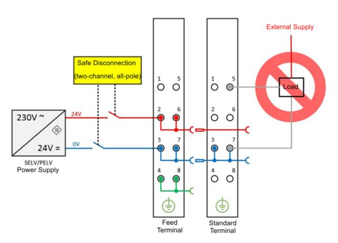
Fig. 1: Negative example - active load
