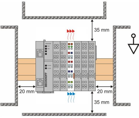
Fig. 19: Recommended distances for standard installation position
