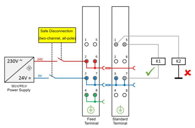
Fig. 2: Ground connection of the load: correct (K1) and incorrect (K2)
