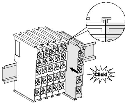
Fig. 12: Attaching on mounting rail
