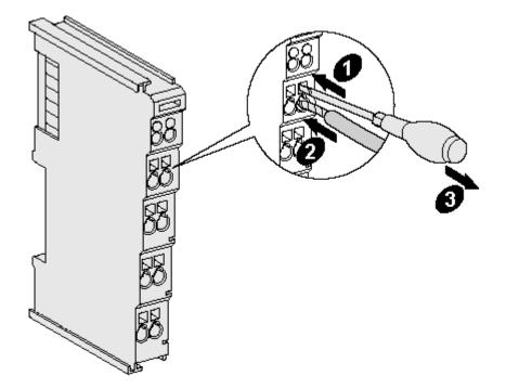
Fig. 18: Mounting a cable on a terminal connection
