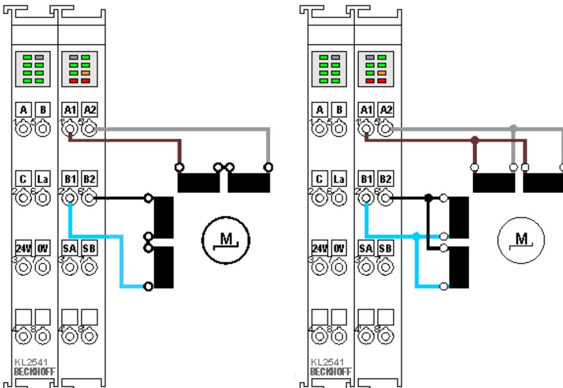
Fig. 25: KL2541 - Bipolar serial (left) and parallel (right) control of a bipolar motor
