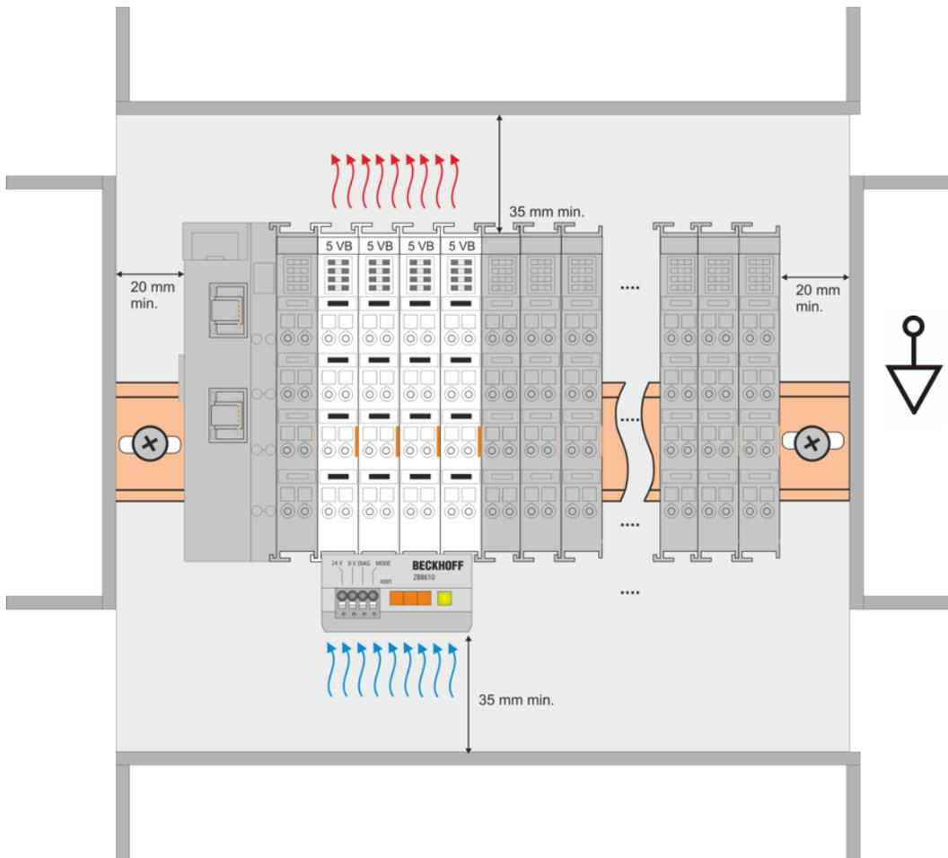
Fig. 14: Recommended distances for installation position for operation with fan
