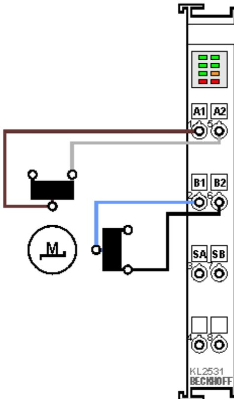
Fig. 23: KL2531 - Bipolar control of a unipolar motor
