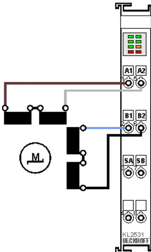
**Bipolar control (parallel) of a bipolar motor**
