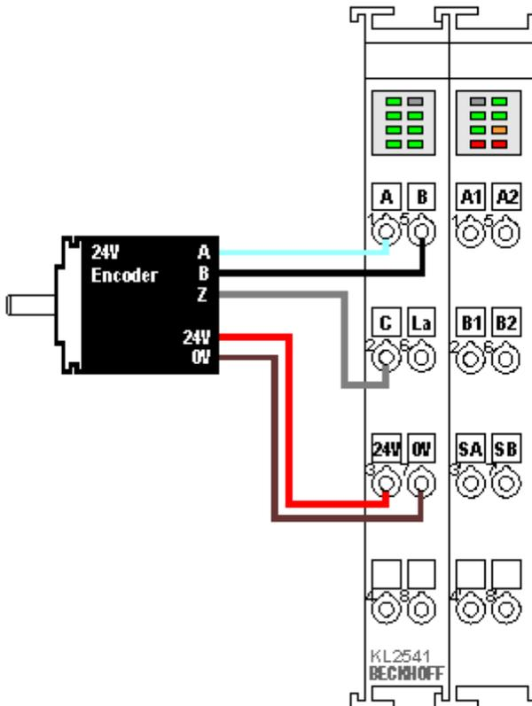
Fig. 27: KL2541 - Connecting an encoder
