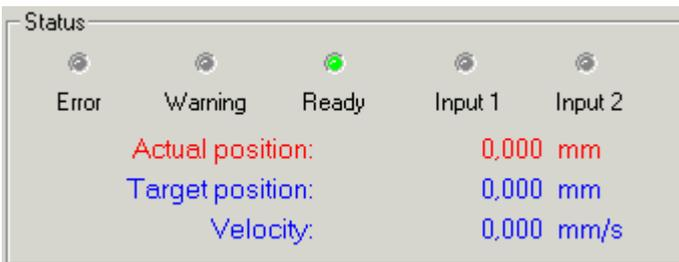
Fig. 40: Status and position display in the *Commissioning* tab
