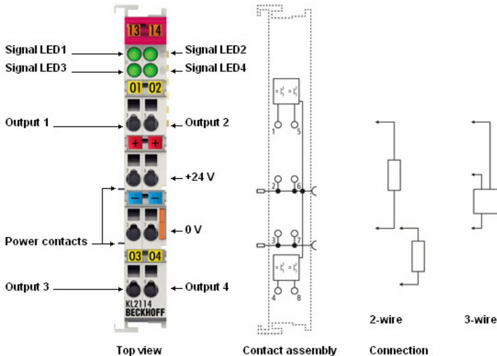
**Four-channel, digital output terminal, 24 V<sub>DC</sub>**
