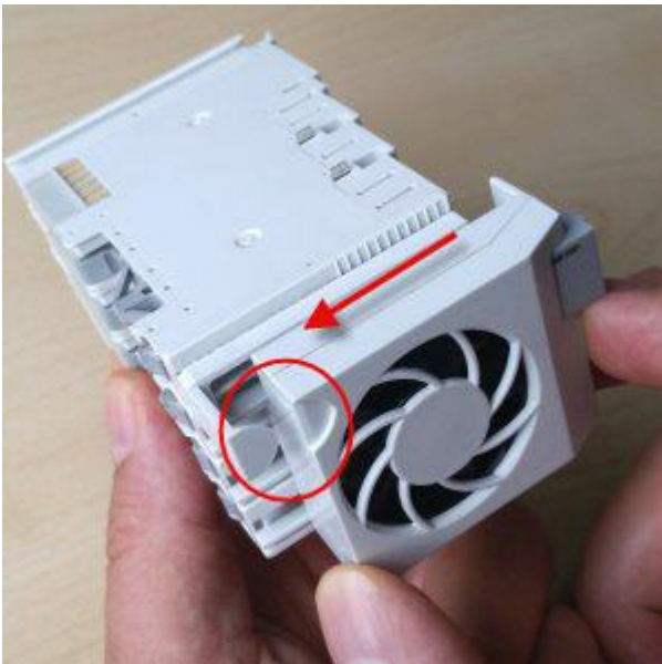
Fig. 9: Push fan cartridge with recess over holding tab
