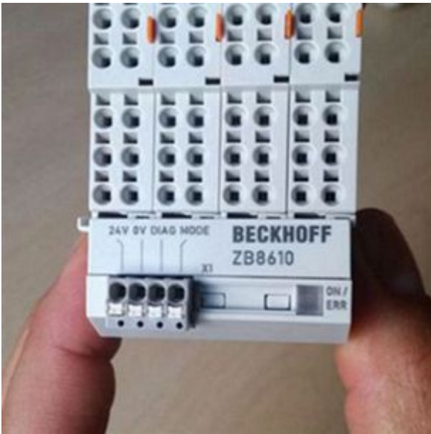
Fig. 11: Correctly attached fan cartridge, front view
