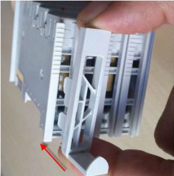
Fig. 5: Engaging the holder for the fan cartridge
