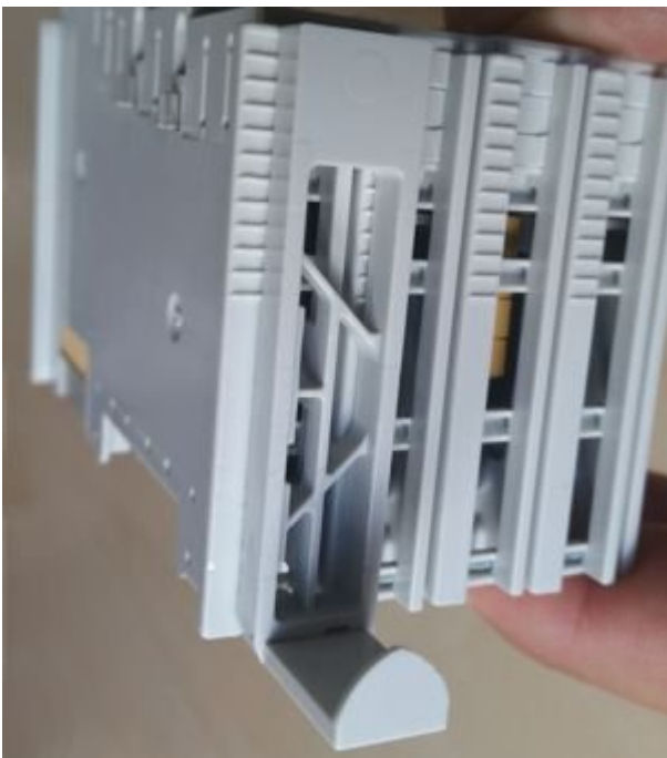
Fig. 6: Correctly engaged holder, front view
