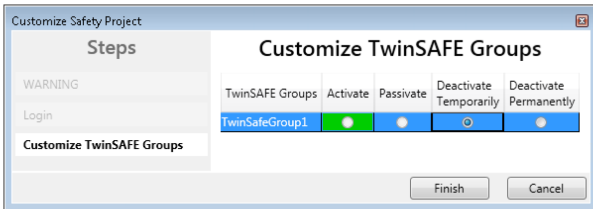
Abb. 168: Customized TwinSAFE Group
