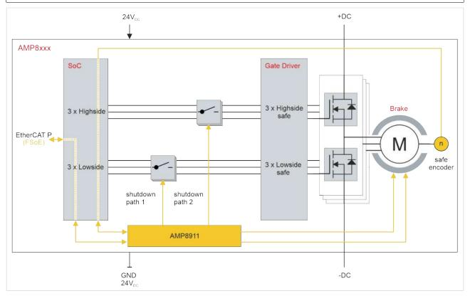
The block diagram describes the mode of operation of the TwinSAFE card within the servo drive.
