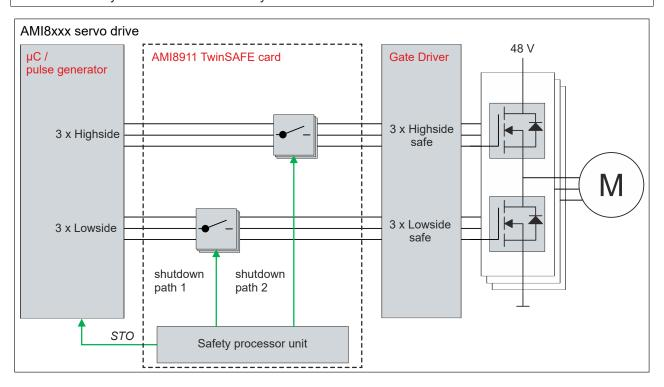
The block diagram describes the mode of operation of the TwinSAFE card within the servo drive.
