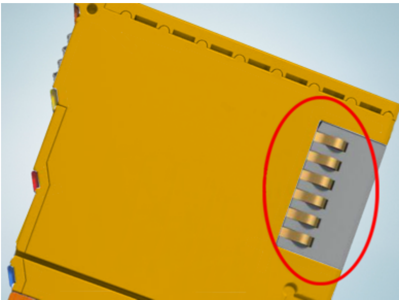
Fig. 6: Spring contacts of Beckhoff I/O components
