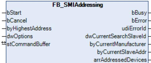
This function block addresses the connected SMI devices according to the random principle. The user has no influence over which address is assigned to which SMI device. The addresses are assigned in descending order, starting with the address specified by the *byHighestAddress* parameter.
