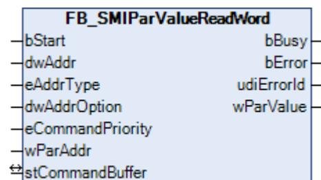
Reads a Word parameter (2 bytes) stored on the motor side. The meaning of the individual parameters is manufacturer-specific.
