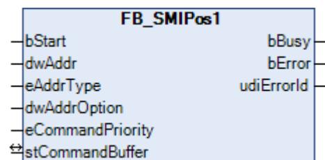
Drives to the fixed position *Pos1* configured on the motor side. The reading and changing of *Pos1* is possible with the [FB\\_SMIPos1Read\(\) \[▶ 23\]](#) and [FB\\_SMIPos1Write\(\) \[▶ 24\]](#) blocks.
