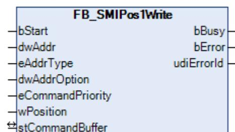
Writes the fixed position *Pos1* which is configurable on the motor side. *Pos1* can be changed using the `FB_SMIPos1Read()` [► 23] block.
