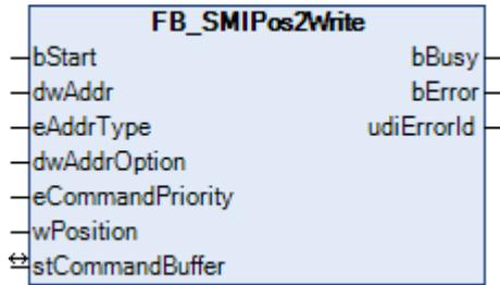
Writes the fixed position *Pos2* which is configurable on the motor side. *Pos2* can be changed using the `FB_SMIPos2Read()` [► 27] block.
