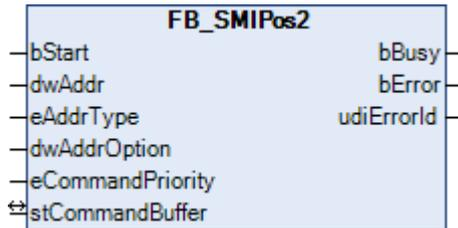
Drives to the fixed position *Pos2* configured on the motor side. The reading and changing of *Pos2* is possible with the [FB\\_SMIPos2Read\(\)](#) [► 27] and [FB\\_SMIPos2Write\(\)](#) [► 28] blocks.
