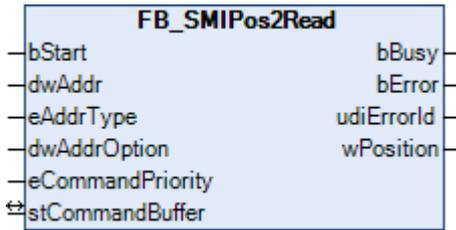
Reads the fixed position *Pos2* configured on the motor side. *Pos2* can be changed using the [FB\\_SMIPos2Write\(\)](#) [▶ 28] function block.
