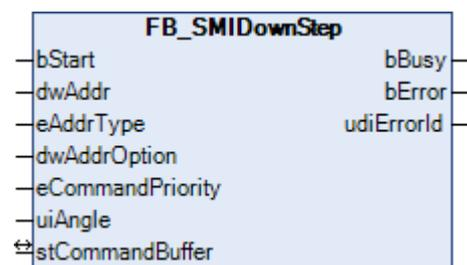
Motor operation downwards by a specified angular degree (0-510 degrees).
