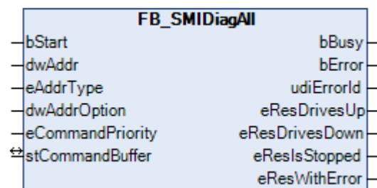
Using this command it is possible to determine the direction in which the drives are driving, whether they have stopped or whether there is a motor error. The command can also be sent also to several SMI slaves. The states of all SMI slaves can thus be queried with a single command.
