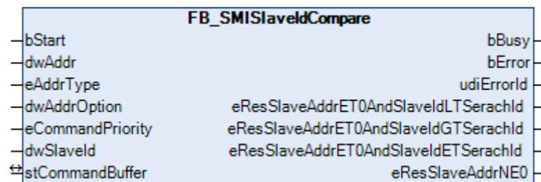
A specified slave ID (32-bit key ID) is compared with the slave ID (32-bit key ID) of one or more drives which is defined on the motor side. The command can also be sent also to several SMI slaves.
