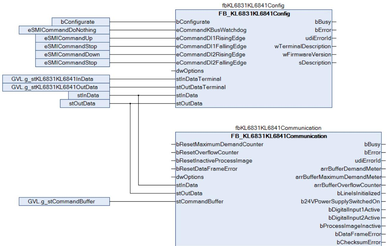
The function block FB\_KL6831KL6841Config() is linked to the process image of the KL6831/KL6841. Once the configuration is complete, the function block FB\_KL6831KL6841Communication() [▶ 12] received the process values of the KL6831/KL6841. No SMI commands can be sent while the configuration is in progress.
