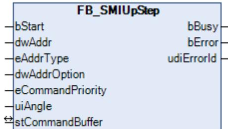
Motor operation upwards by a specified angle (0-510 degrees).
