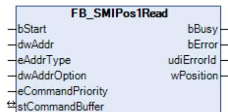
Reads the fixed position *Pos1* configured on the motor side. *Pos1* can be changed using the FB\_SMIPos1Write() [▶ 24] function block.
