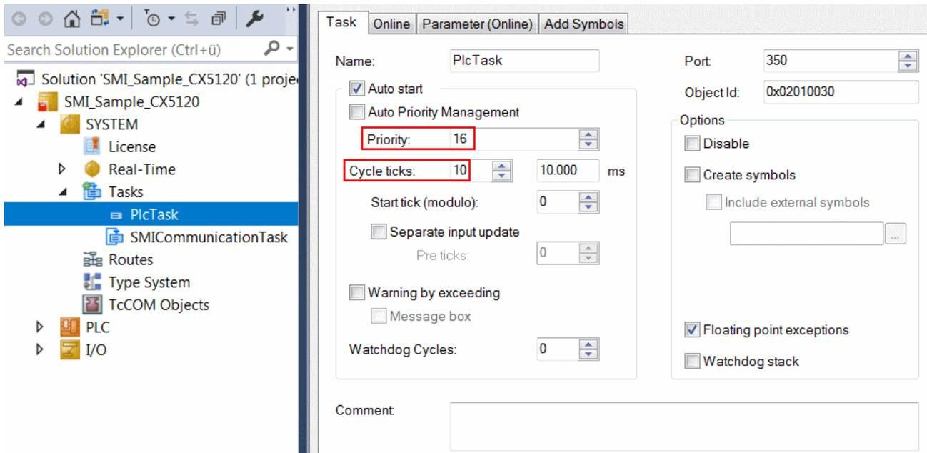
Create a further task for the background communication. Assign a higher priority (smaller number) and a lower interval time to this task than the PlcTask.
