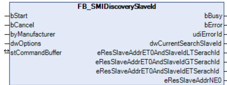
The first drive is sought that corresponds to the specified manufacturer code and has the address 0. This function block is used in the addressing of SMI devices and is used in the FB\_SMIAddressing() [▶ 35] function block.
