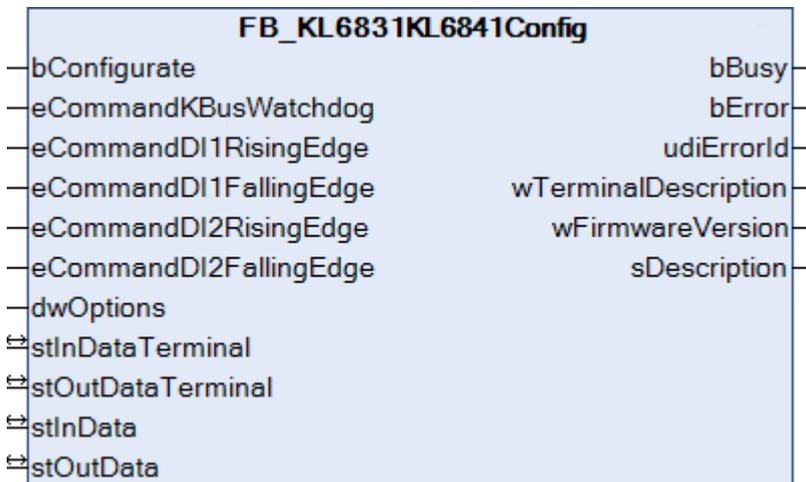
This function block is used to configure the KL6831/KL6841. The configuration is executed when the PLC program starts, or it can be triggered by a positive edge at the input *bConfigurate*. The parameters are stored in the respective registers of the KL6831/KL6841 in a non-volatile manner. In addition, some general information, such as the firmware version, is read from the KL6831/KL6841.
