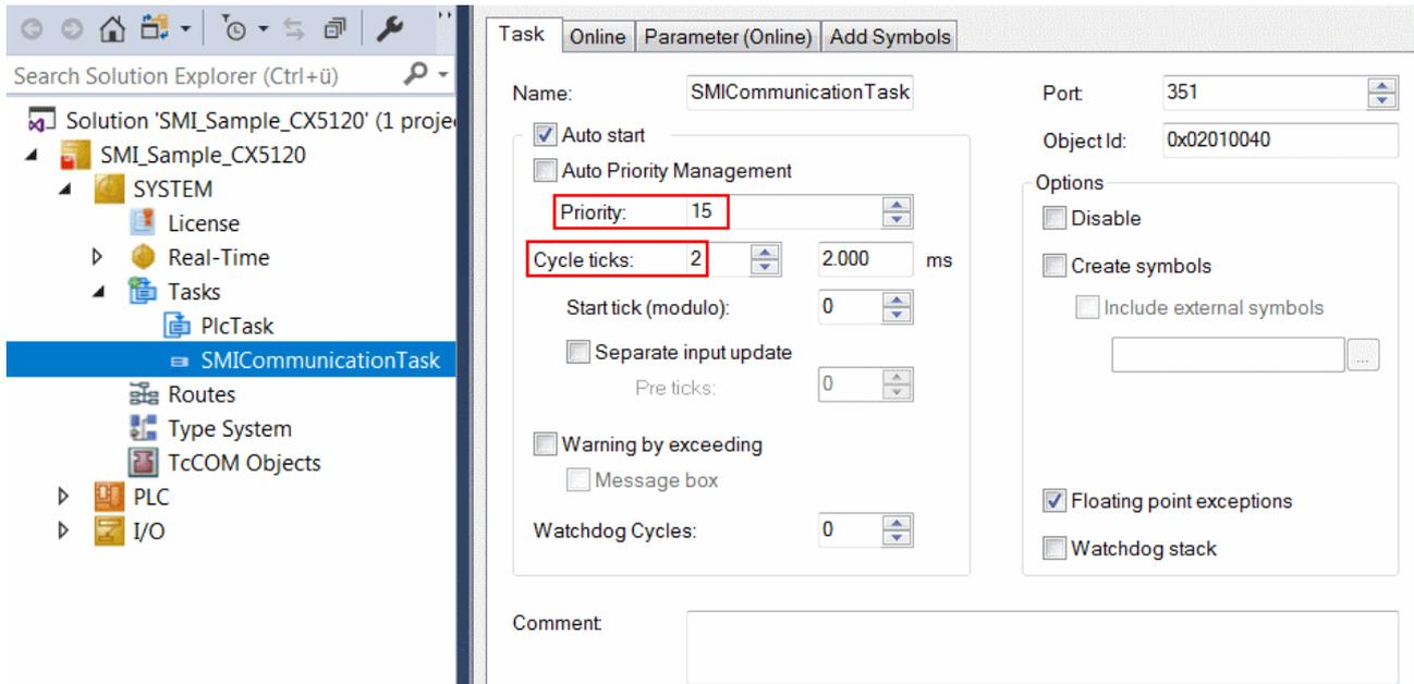
Add the program for the communication to this task. More precise information on the task configuration can be found in the function block description.
