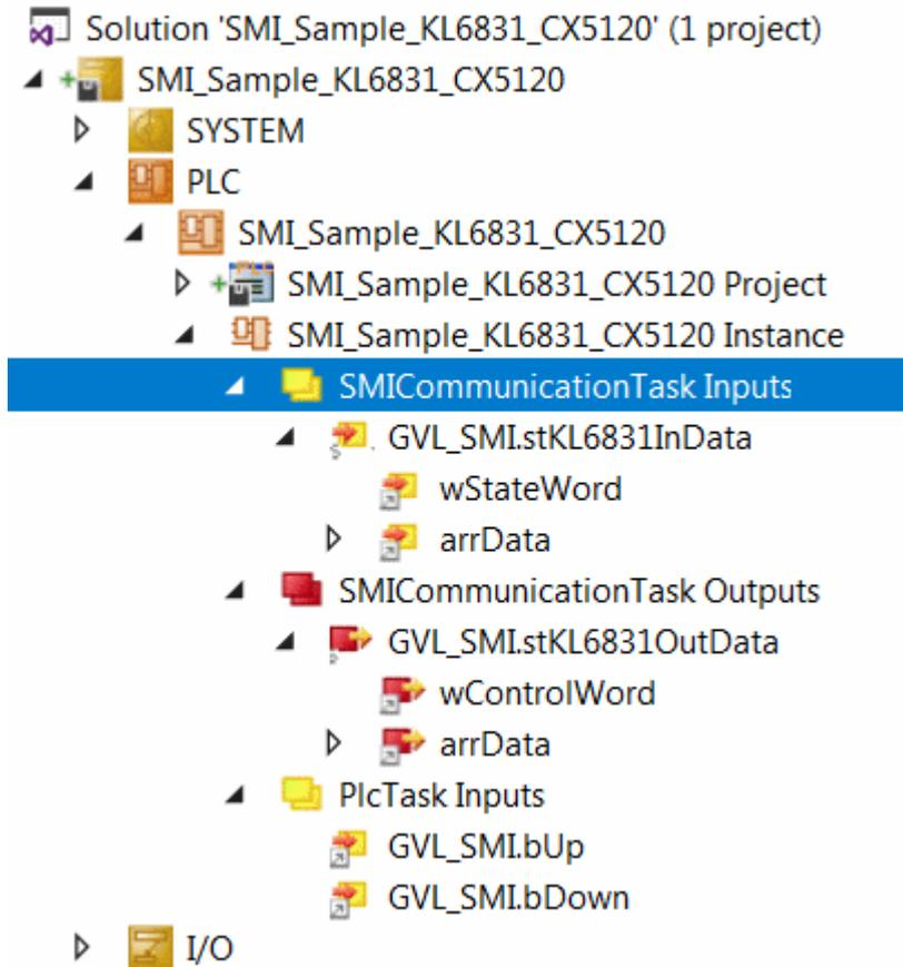
Now link the global variables of PLC program with the inputs and outputs of the Bus Terminals. Create the Solution and enable the configuration.
