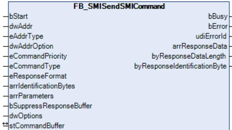
This function block is for the general sending of an SMI command. The precise structure of an SMI command and the functioning of the KL6831/KL6841 must be known for this. The use of this function block is necessary only if an SMI command is to be sent that is not covered by the other PLC function blocks.
