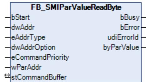
Reads a byte parameter (1 byte) stored on the motor side. The meaning of the individual parameters is manufacturer-specific.
