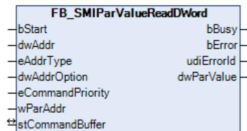
Reads a DWord parameter (4 bytes) stored on the motor side. The meaning of the individual parameters is manufacturer-specific.
