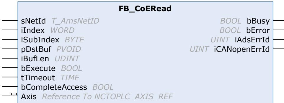
The function block FB\_CoERead allows data to be read from an object directory of an EtherCAT slave through an SDO (Service Data Object) access. This requires the slave to have a mailbox and to support the CoE (CANopen over EtherCAT) protocol. With the help of the SubIndex and Index parameters a selection is made as to which object should be read out. Via CompleteAccess := TRUE the parameter can be read with sub-elements.
