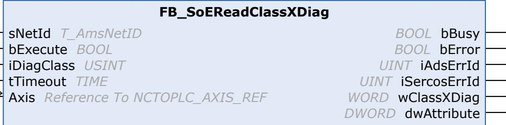
With the function block FB\_SoEReadClassXDiag, the current Class 1 diagnosis (S-0-0011) ... Class 3 diagnosis (S-0-0013) can be read out as WORD. There is the conversion function F\_ConvWordToSTAX5000C1D for the evaluation of the Class 1 diagnosis as a structure ST\_AX5000\_C1D, (see TwinCAT 3 PLC Lib Tc2\_Drive documentation).
