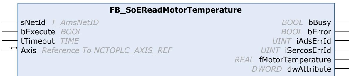
With the function block FB\_SoEReadMotorTemperature the temperature of the motor (S-0-0383) can be read. If the motor does not contain a temperature sensor, this is 0.0, i.e. 0.0 °C.
