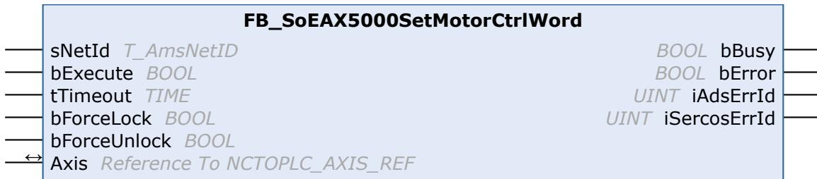
With the function block FB\_SoEAX5000SetMotorCtrlWord the ForceLock bit (Bit 0) or the ForceUnlock bit can be set in the Motor Control Word (P-0-0096) to activate or release the brake. Normally the brake is automatically controlled via the Enable of the drive.
