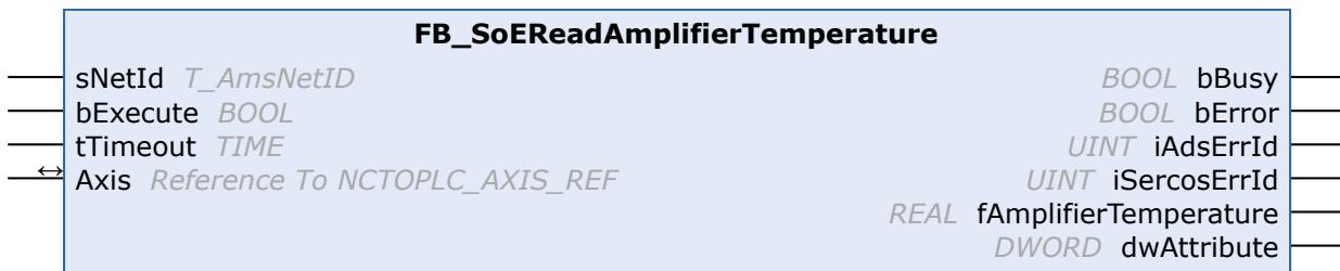
With the FB\_SoEReadAmplifierTemperature function block the temperature of the drive (S-0-0384) can be read.
