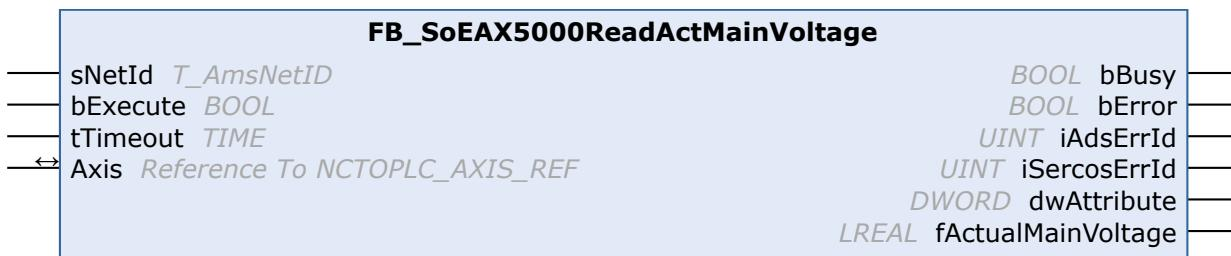
With the FB\_SoEAX5000ReadActMainVoltage function block the current peak value of the mains voltage of the AX5000 (P-0-0200) can be read.
