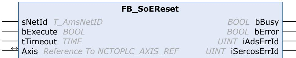
The drive (S-0-0099) can be reset with the function block FB\_SoEReset. In the case of multiple-channel devices if necessary, both channels will have to perform a reset. The timeout time must be 10 s, as the reset can take up to 10 s depending on the error. The flag "Wait For WcState is OK" must be enabled in the advanced EtherCAT settings for the AX5000.
