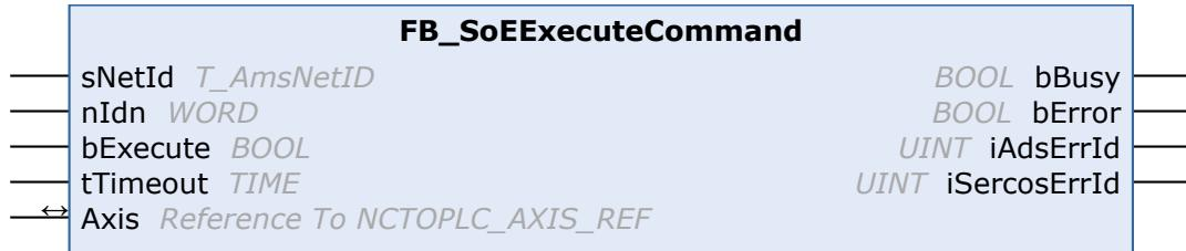
With the FB\_SoEExecuteCommand function block a command can be executed.
