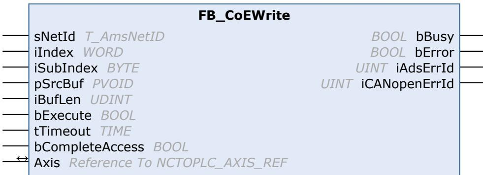
With the function block FB\_CoEWrite, an object from the object directory of an EtherCAT slave can be written via an SDO (Service Data Object) download. This requires the slave to have a mailbox and to support the CoE (CANopen over EtherCAT) protocol. With the help of the SubIndex and Index parameters a selection is made as to which object should be written. Via CompleteAccess := TRUE the parameter can be written with sub-elements.
