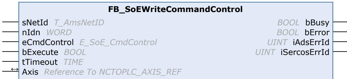
With the FB\_SoEWriteCommandControl function block a command can be prepared, started or canceled.
