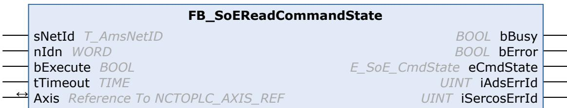
With the FB\_SoEReadCommandState function block the command execution can be checked.
