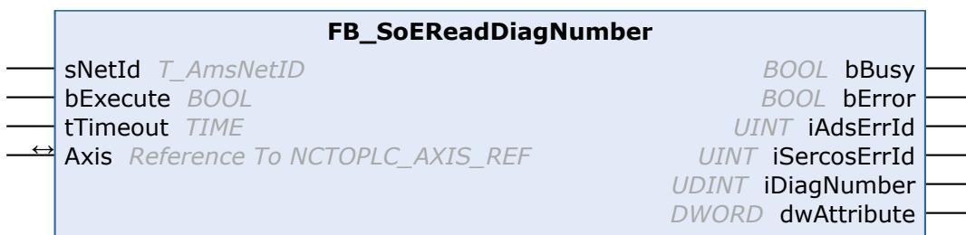
With the FB\_SoEReadDiagNumber function block the current diagnostic number can be read out as UDINT (S-0-0390).
