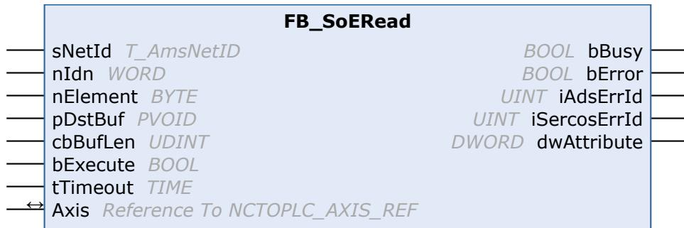
With the FB\_SoERead function block a parameter can be read.
