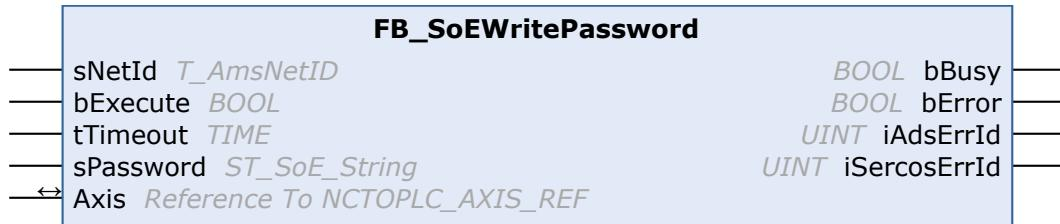
With the FB\_SoEWritePassword function block (S-0-0267) the drive password can be set.
