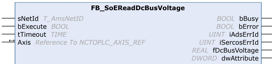
With the FB\_SoEReadDcBusVoltage function block the Dc-Bus voltage of the drive (S-0-0380) can be read.
