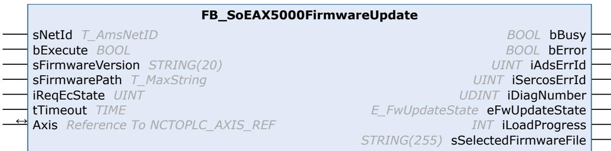
With the FB\_SoEAX5000FirmwareUpdate function block the Firmware of the AX5000 can be checked and automatically changed to a given version (Revision and Build) or to the current Build of the configured revision.
