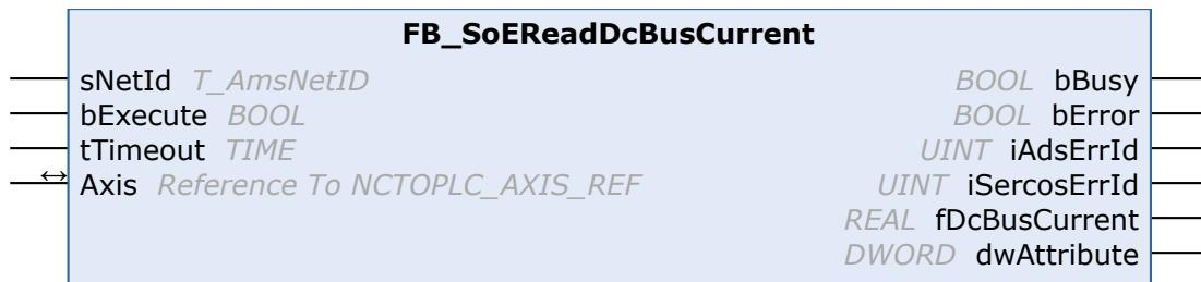
With the function block FB\_SoEAX5000ReadDcBusCurrent the DC-Bus current (S-0-0381) can be read.
