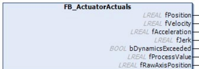
This core function is used to display a compilation of actual values of an actuator. It is an extension of Actuals and extends the range of its parent element by adding specific interpretations for actuators.
