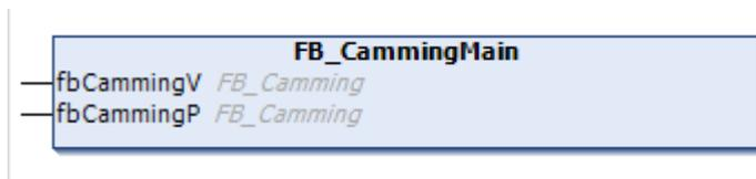
The property provides two options: Camming.Pos for position camming and Camming.Velo for velocity camming. To do this, two classes of the same type are instantiated, but with different parameterizations.
