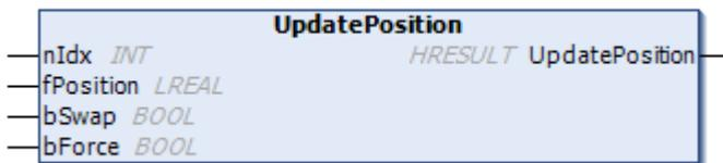
In some use cases, the target position of the segments must be modified after definition. This method is used for transforming axes, for example.
