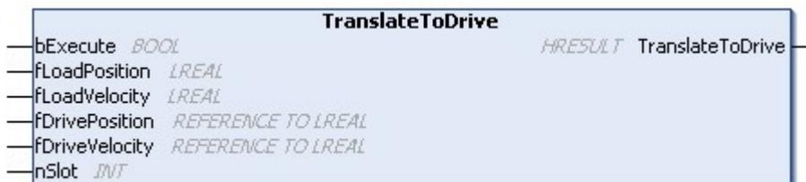
This method is used to calculate a drive position using the transformation table of the load table.
