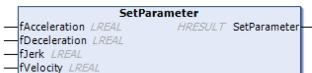
This method is used to set the parameters of a movement in jogging mode.
