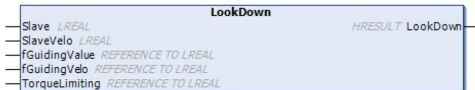
This method translates a slave value to a matching master value. If the value lies between two defined points in the table, the selected operation mode is used for interpolation.
