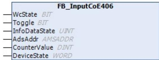
This class can be used for a DS406 based encoder. In this context, the term CoE (CAN over EtherCAT) refers to the transmission of the CiA DS406 protocol via EtherCAT.
