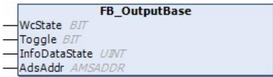
This class is the basis for I/O output elements.
