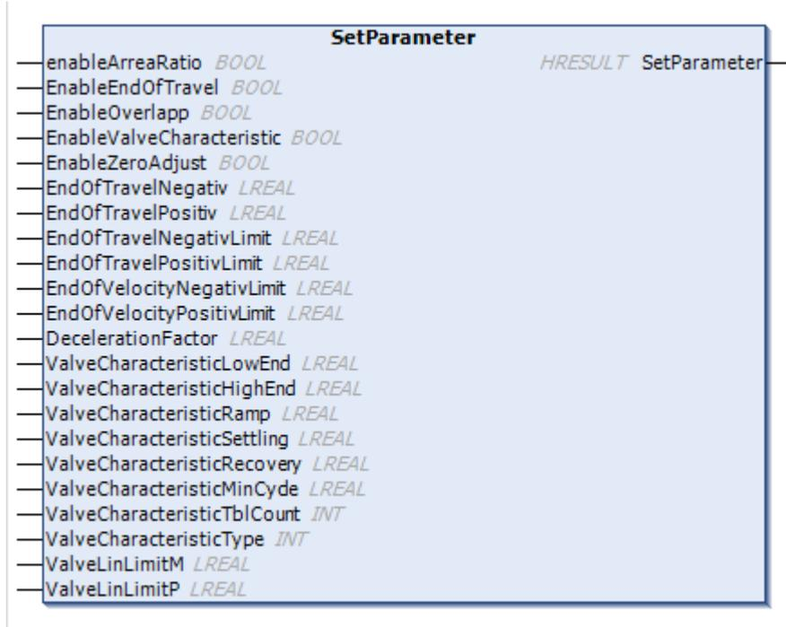
This method can be used to set the parameters for identification.
