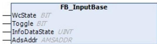
This class is the basis for I/O input elements.
