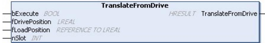
This method is used to calculate a load position using the transformation table of the load table.
