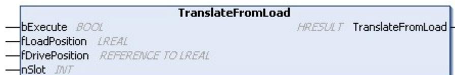
This method is used to calculate a drive position using the transformation table of the drive side.
