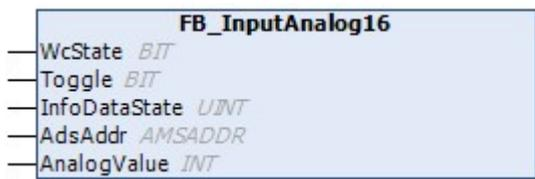
This class can be used for a 16-bit analog input element.
