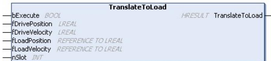
This method is used to calculate a load position via the transformation table of the drive side.
