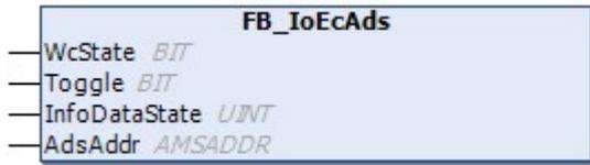
This class is the basis for EtherCAT-based I/O elements with ADS interface.
