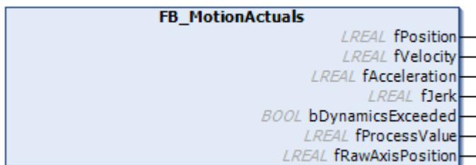
This core function is not instantiated directly. It is used as a common part of type-specific core functions like ActualsHydraulics, ActualsNc or ActualsActuator.
