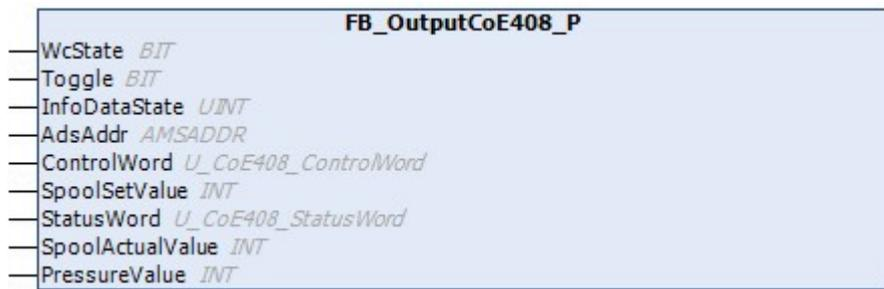
This class is an extension of the CoE408-based valve with integrated pressure measurement.
