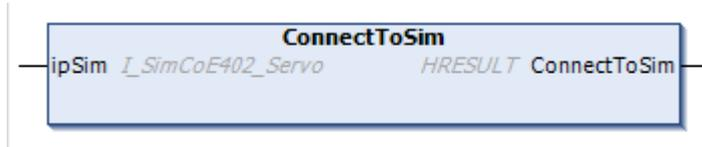
This method establishes a connection between the torque-limiting FB and the simulated servo drive. This connection replaces the EtherCAT communication with a real CoE402-based servo drive.
