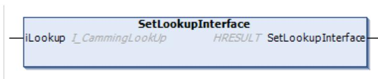
This method must be used to connect a camming table.
