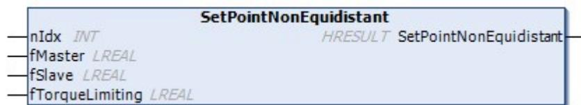
This method sets a point in the table addressed via `nIdx` that has a specific master position. To do this, the table must be initialized in a non-equidistant operation mode.
