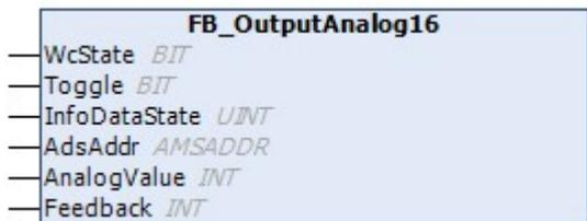
This class can be used for a 16-bit analog output element.
