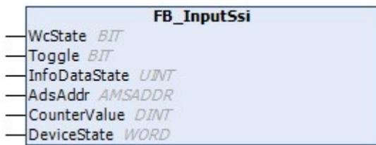
This class can be used for an SSI based encoder.
