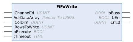
The function block FiFoWrite reads position data for *iColDim* FIFO channel axes from *AdrDataArray* and transfers *iRowsToWrite* entries to the FIFO.
