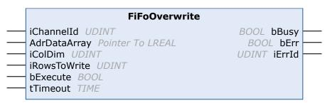
The function block FiFoOverwrite reads position data for *iColDim* FIFO channel axes from *AdrDataArray* and transfers *iRowsToWrite* entries to the FIFO. Existing FIFO data will be overwritten.
