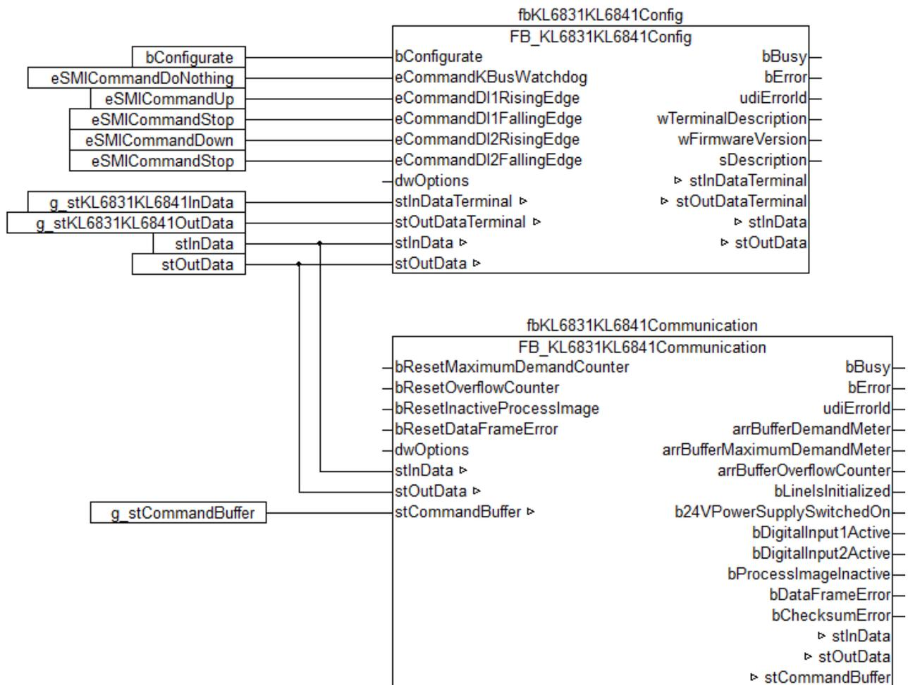
The block FB\_KL6831KL6841Config() is linked to the process image of the KL6831/KL6841. After the configuration, the block FB\_KL6831KL6841Communication() is assigned the process values of the KL6831/KL6841. During the configuration, it is not possible to send SMI commands.
