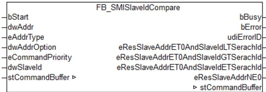
A specified slave ID (32-bit key ID) is compared with the slave ID (32-bit key ID) of one or more drives which is defined on the motor side. The command can also be sent also to several SMI slaves.
