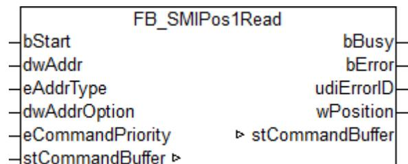
Reads the fixed position *Pos1* configured on the motor side. *Pos1* can be changed using the `FB_SMIPos1Write()` [▶ 32] block.
