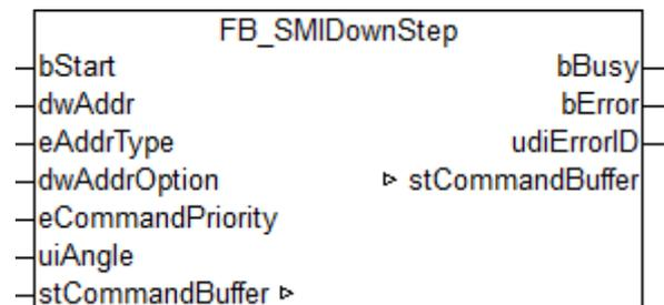
Motor operation downwards by a specified angular degree (0-510 degrees).
