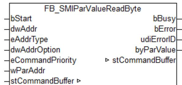
Reads a byte parameter (1 byte) stored on the motor side. The meaning of the individual parameters is manufacturer-specific.
