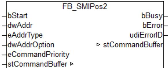
Drives to the fixed position *Pos2* configured on the motor side. The reading and changing of *Pos2* is possible with the [FB\\_SMIPos2Read\(\)](#) [▶ 34] and [FB\\_SMIPos2Write\(\)](#) [▶ 35] blocks.
