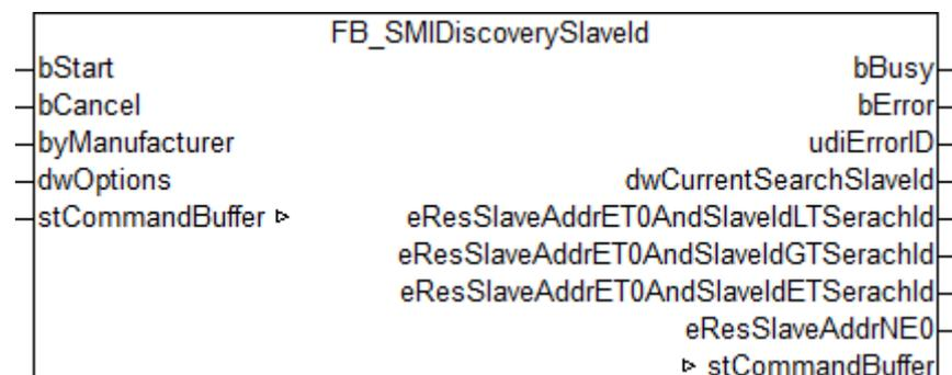
The first drive is sought that corresponds to the specified manufacturer code and has the address 0. This function block is used in the addressing of SMI devices and is used in the [FB\\_SMIAddressing \[▶ 42\]](#) block.
