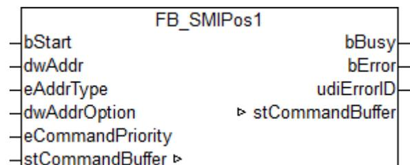
Drives to the fixed position *Pos1* configured on the motor side. The reading and changing of *Pos1* is possible with the `FB_SMIPos1Read()` [▶ 30] and `FB_SMIPos1Write()` [▶ 32] blocks.
