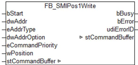
Writes the fixed position *Pos1* which is configurable on the motor side. *Pos1* can be changed using the `FB_SMIPos1Read()` [▶ 30] block.
