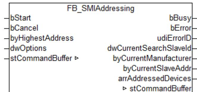
This function block addresses the connected SMI devices according to the random principle. The user has no influence over which address is assigned to which SMI device. The addresses are assigned in descending order, starting with the address specified by the *byHighestAddress* parameter.
