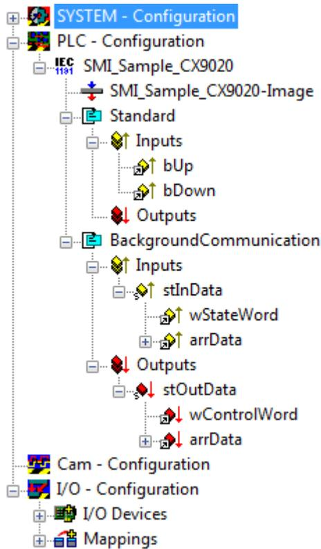
Now link the global variables of the PLC program with the Bus Terminal inputs and outputs, create the allocations, and activate the configuration. Then start the device in run mode. Your CX is now ready for use.
