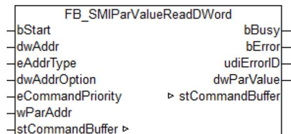
Reads a DWord parameter (4 bytes) stored on the motor side. The meaning of the individual parameters is manufacturer-specific.
