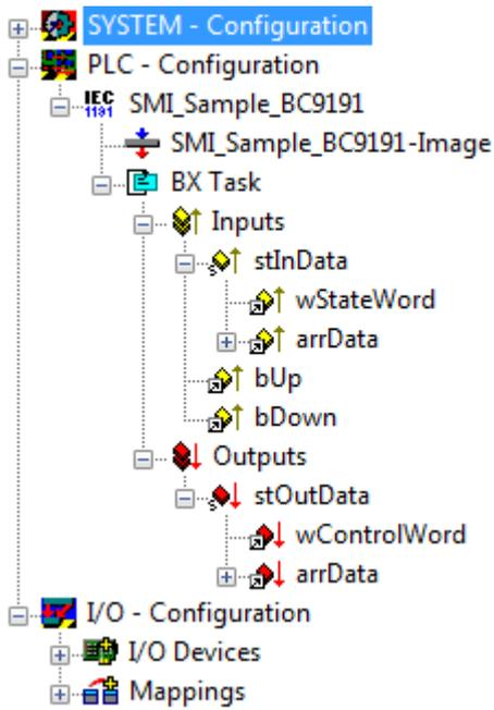
Now link the global variables of the PLC program with the Bus Terminal inputs and outputs, create the allocations, and activate the configuration. Then start the device in run mode. Your BC is now ready for use.
