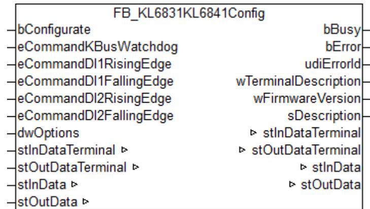
This block is used to configure the KL6831/KL6841. The configuration is executed when the PLC program starts, or it can be triggered by a positive edge at the input *bConfigure*. The parameters are stored in the respective registers of the KL6831/KL6841 in a fail-safe manner. In addition, some general information, such as the firmware version, is read from the KL6831/KL6841.
