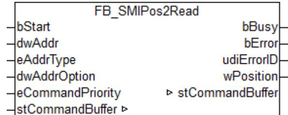
Reads the fixed position *Pos2* configured on the motor side. *Pos2* can be changed using the `FB_SMIPos2Write()` [► 35] block.
