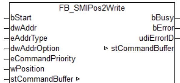
Writes the fixed position *Pos2* which is configurable on the motor side. *Pos2* can be changed using the `FB_SMIPos2Read()` [\[► 34\]](#) block.
