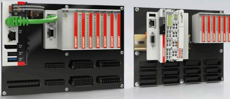
Various Industrial and Embedded PCs can also be integrated directly into the signal distribution board.
