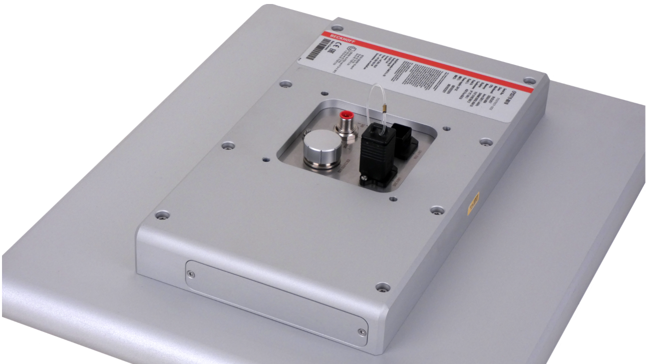
Fig. 2: CFast card slot and battery of the system clock behind the cover plate
