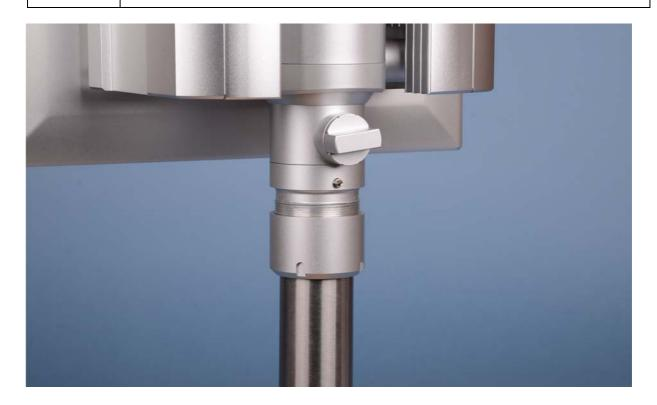
3. Tighten the Allen locking screw using the Allen key (2).
