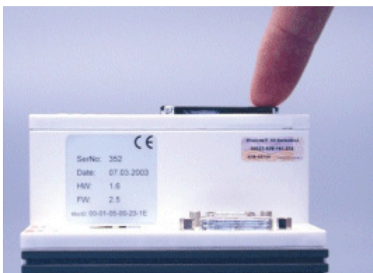
FIG1: Ejecting the CF card
